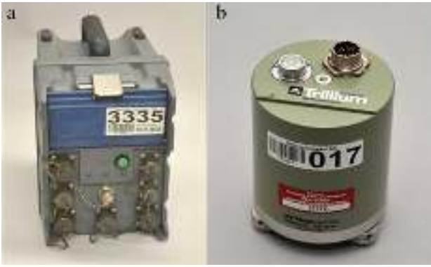
Figure 3. Broadband portable seismic stations deployed during the experiment. (a) EarthData PR6-24 three-channel recorder, and (b) Trillium Compact broadband three-component sensor.
